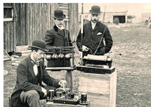
British Post Office engineers inspect Marconi's radio equipment during a demonstration on Flat Holm Island, 13 May 1897. The transmitter center, the coherer receiver below it, pole supporting wire antenna top.
